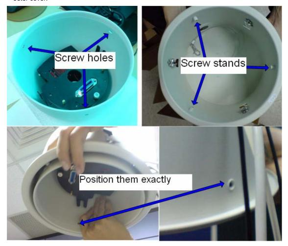
7. Check speed dome main body. Fit in the pin into pin hole of base plate. Drive 2pcs screws until the speed dome fits the plate tightly and solidly
